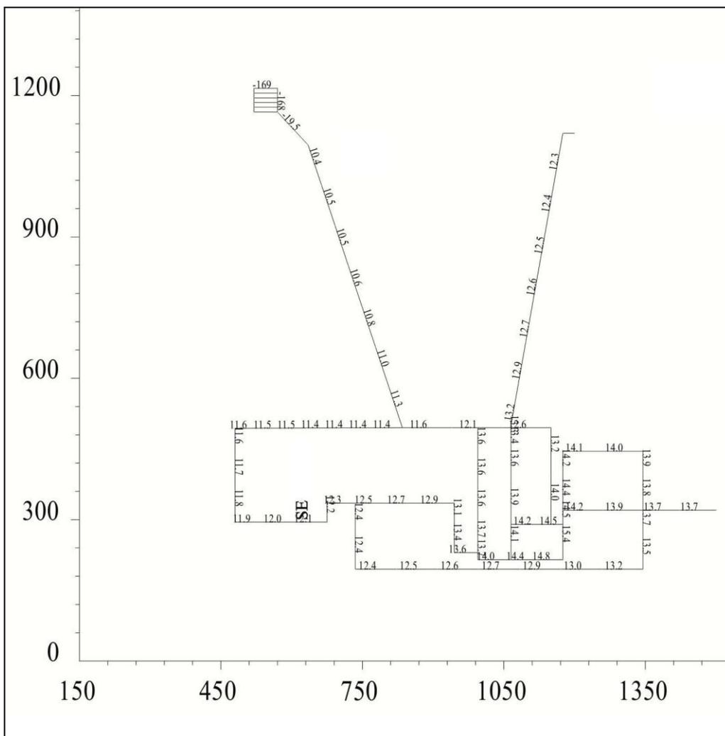
Figure 5.2: industrial grounding grid.
