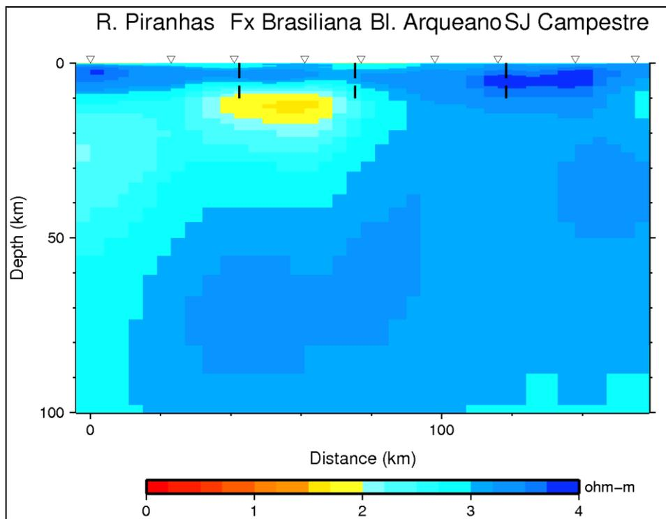
Figure 4.2: 2D soil resistivity profile measured by INPE at Brazil Northeast, along a path 160km long, down to 100km deep (resistivity scale is logarithmic base 10, what means it goes from 1 to 10.000 Ω.m).
