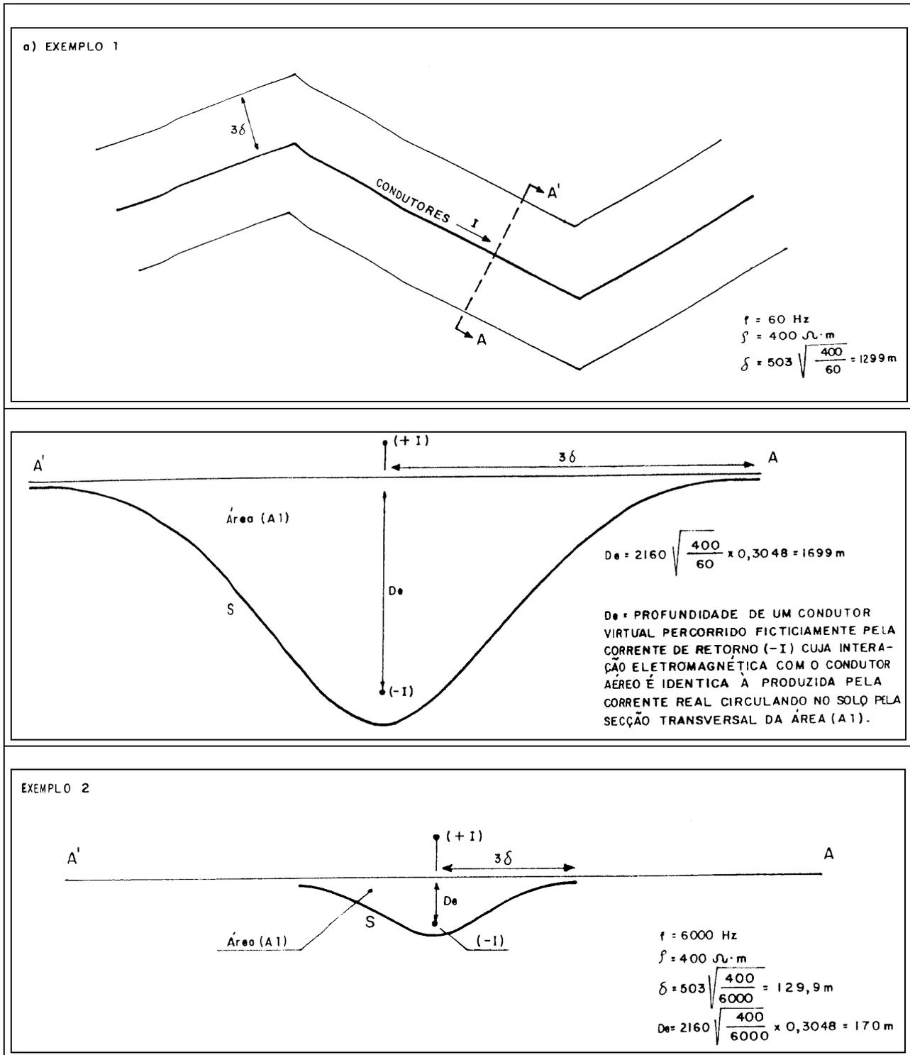
Figure 3.1: circulating pattern of transmission line ground return current.
