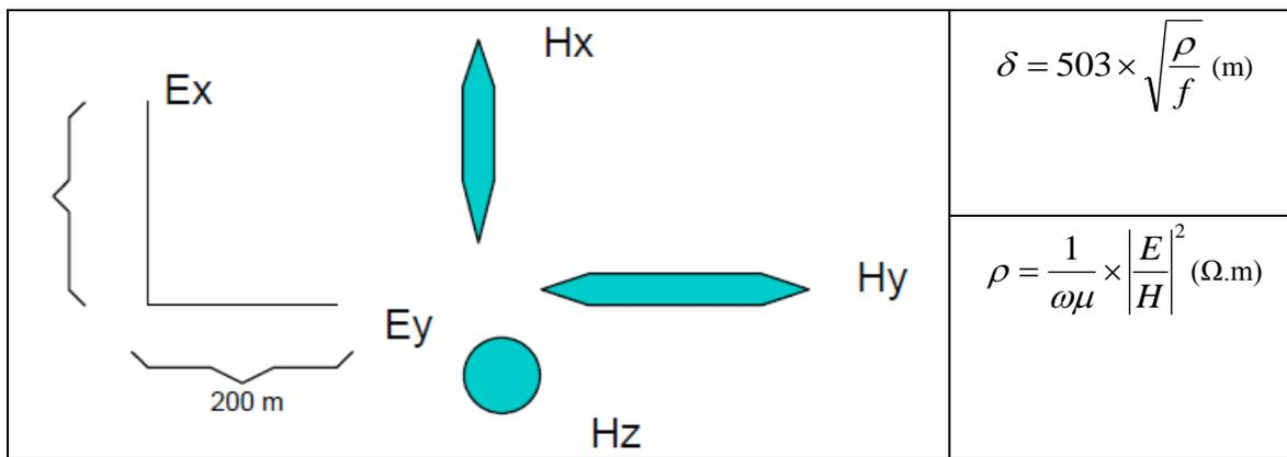
Figure 4.1: MT coils and probes arrangement, for measuring magnetic and electric fields on soil surface, and expressions for the calculation of soil resistivity ( $\rho$ ) and depth of penetration ( $\delta$ ).
