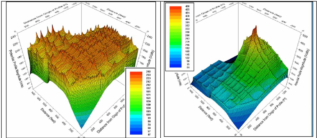
Figure 5.1: soil surface potential profile above a ground mat (360 x 60 m) with two different simulation conditions:
